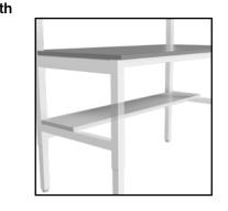
The lower shelf is installed across the bench's lower support.
