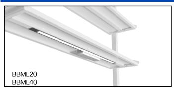
LED Task Lighting consists of a thin-profile, white, LED strip, 9.5 mm high by 33mm deep with a touch dimmer switch. It is UL listed and furnished with a 120 VAC to 24 VDC power supply with ten foot power cord. The light includes a magnetic mounting strip for mounting to steel shelving.
