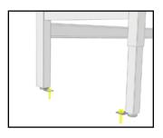
The leg anchor bracket captures the glide on each leg to prevent movement in any direction. The bracket has a mounting hole for an anchor bolt (not included).
