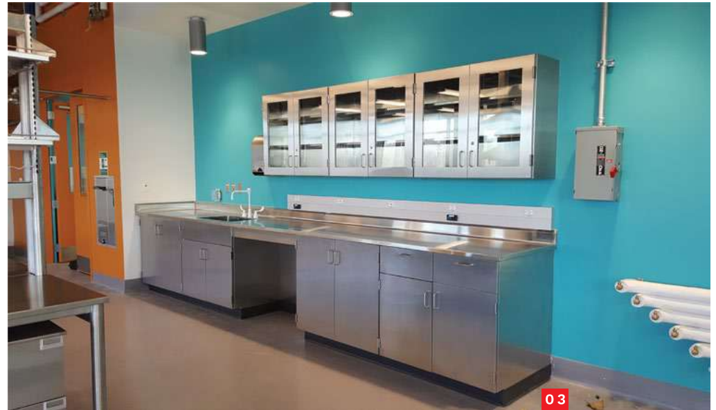
02 Stainless steel Enterprise shared frame bench system with pre-wired electric outlets, task lighting, adjustable-height stainless steel bench work surface shelving, Research Collection full-overlay style stainless steel mobile cabinets with label holders.
