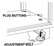
(accessible thru cabinet bottom with straight blade screw driver)
