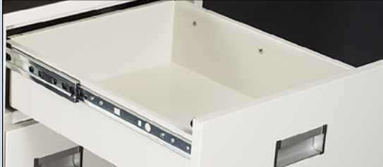
Standard Drawers feature one-piece drawer body construction with full-extension, side mounted, soft-close, slides. (model F-8400-01)
