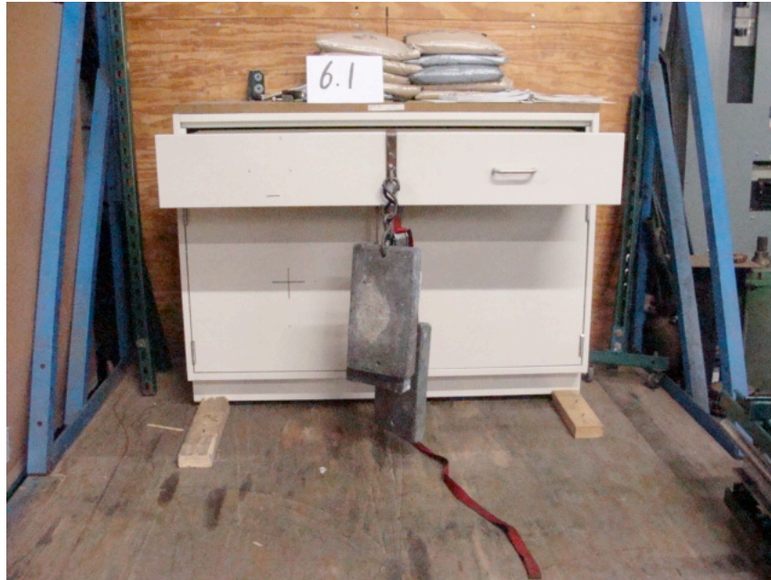
Photo 7: 6.1 Drawer Static Test
