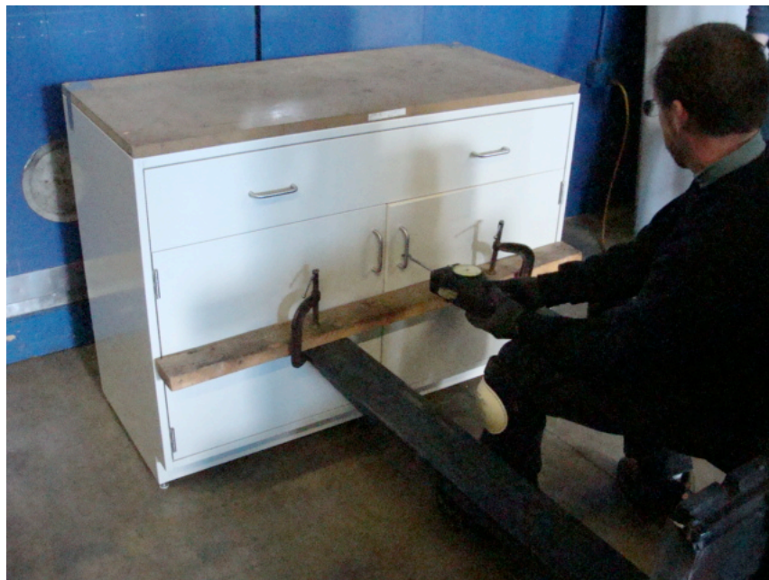
Photo 8: 6.2 Drawer and Door Pull Test
