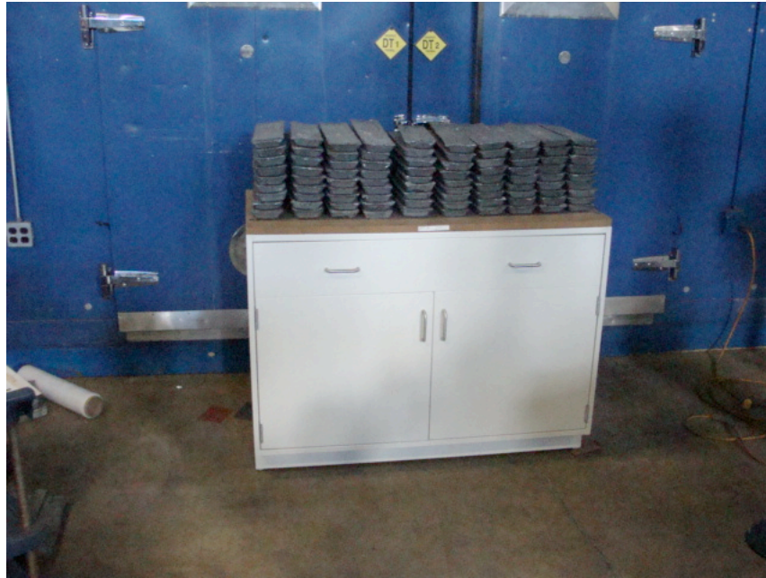
Photo 1: 4.2 Cabinet Load Test
