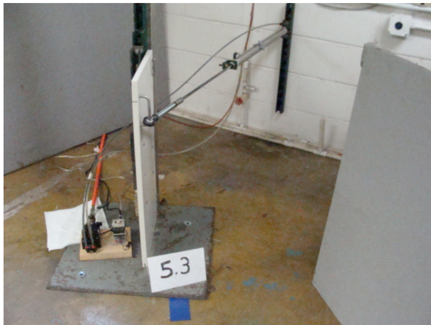
Photo 6: 5.3 Door Cycle Test
