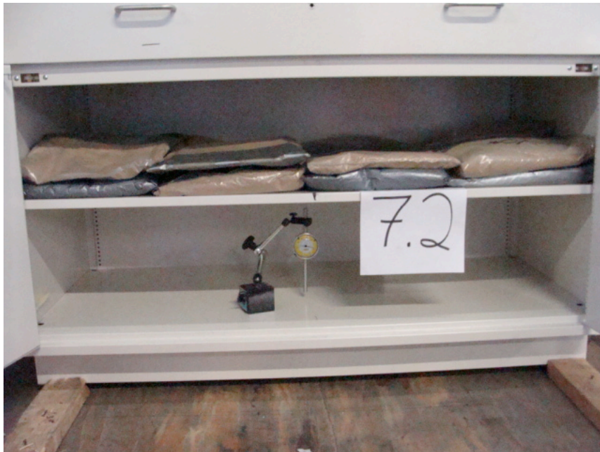
Photo 12: 7.2 Shelf Load Test, 0.238" Deflection
