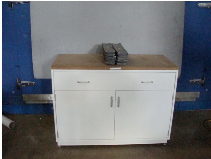
Photo 2: 4.3 Cabinet Concentrated Load Test
