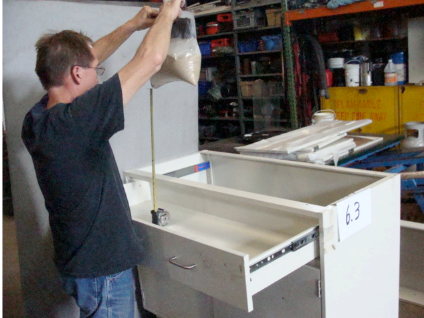
Photo 9: 6.3 Drawer Impact Test
