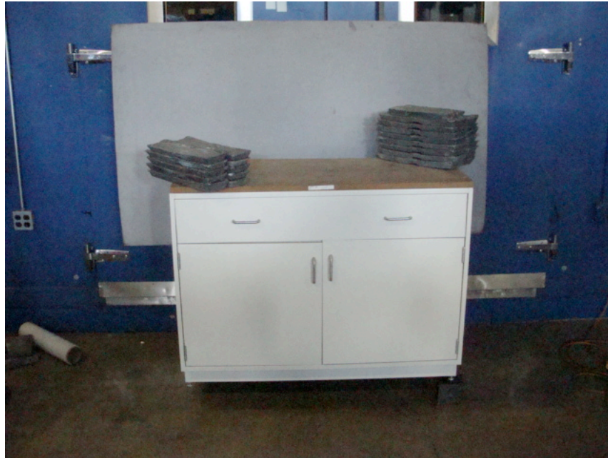
Photo 3: 4.4 Cabinet Torsion Test
