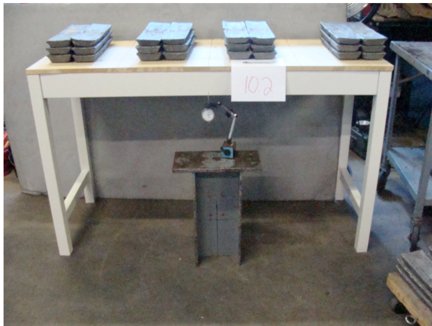
Photo 14: 10.2 Table Static Load
