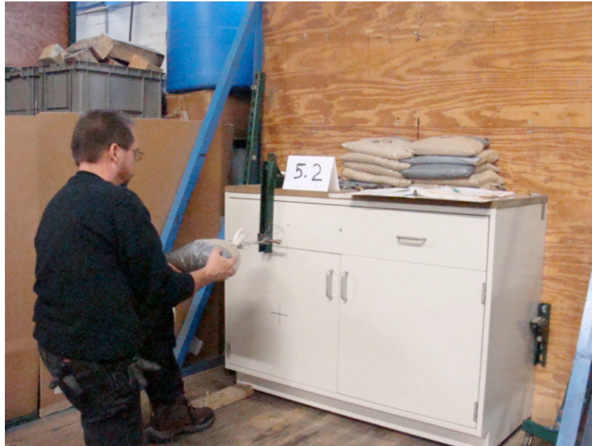
Photo 5: 5.2 Door Impact Test
