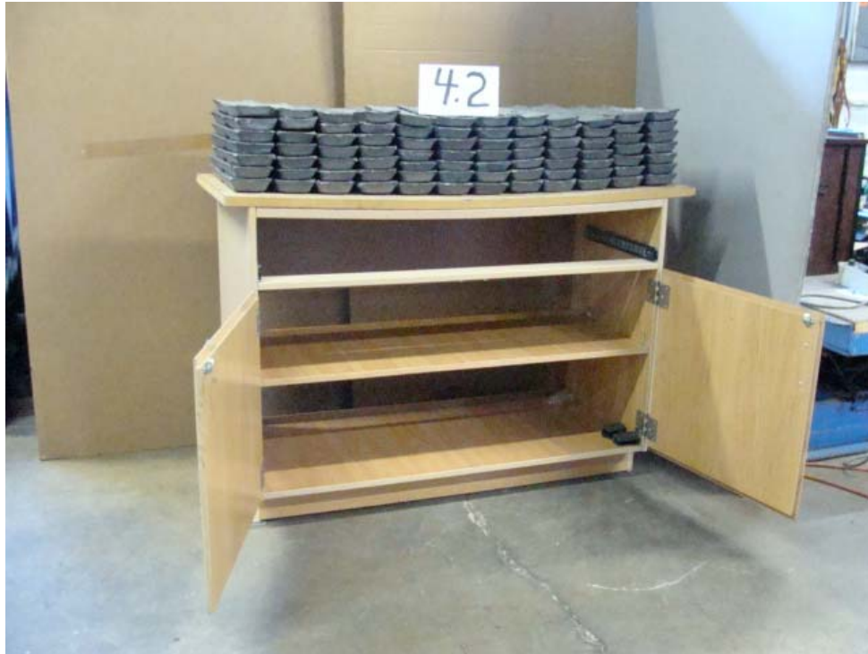
Photo 1: 4.2 Cabinet Load Test
