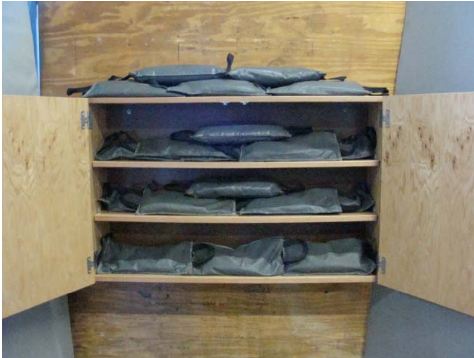
Photo 13: 9.2 Wall Cabinet Load Test
