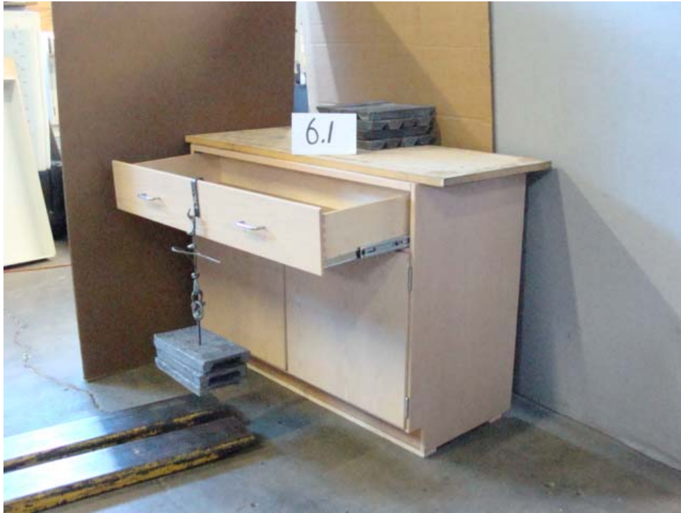
Photo 7: 6.1 Drawer Static Test
