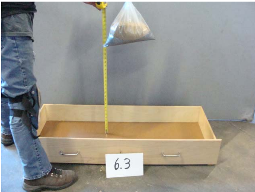
Photo 8: 6.3 Drawer Impact Test
