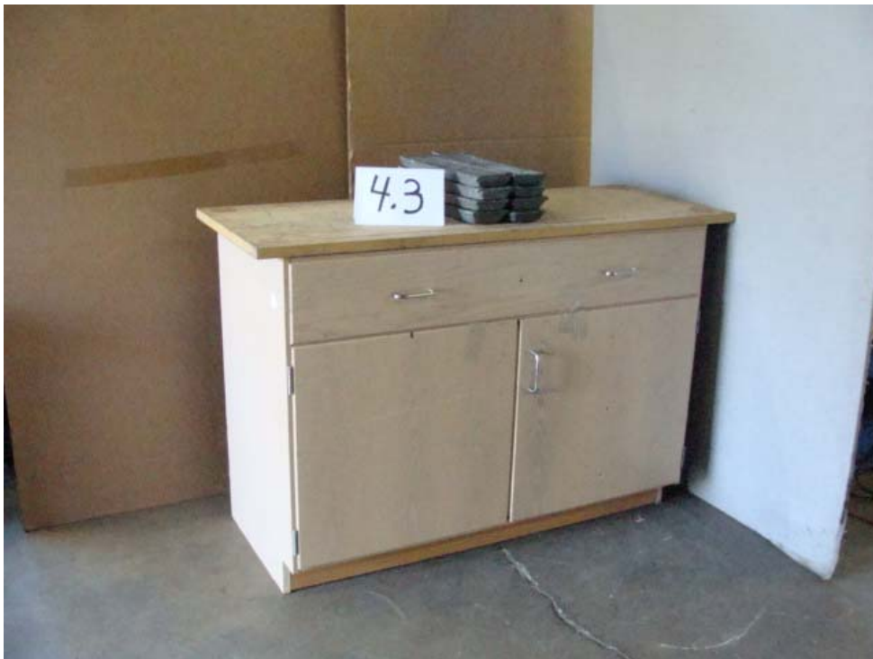
Photo 2: 4.3 Cabinet Concentrated Load Test
