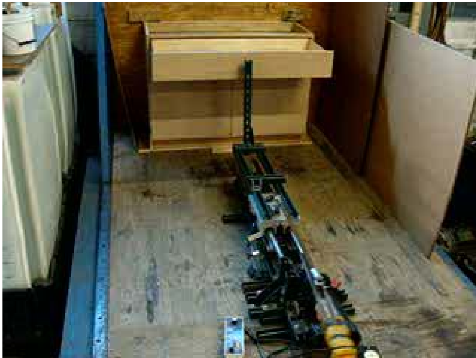
Photo 10: 6.5 Drawer Cycle Test
