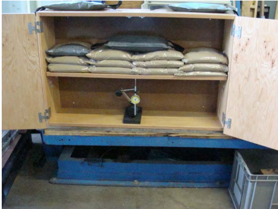
Photo 11: 7.2 Shelf Load Test
