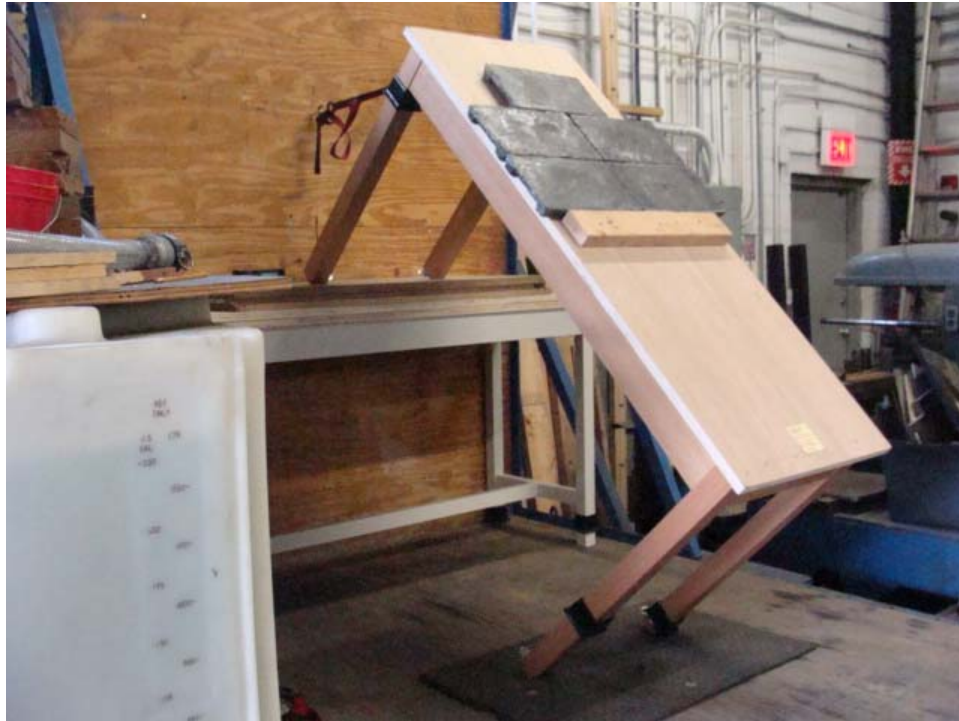
Photo 15: 10.3 Table Racking Test
