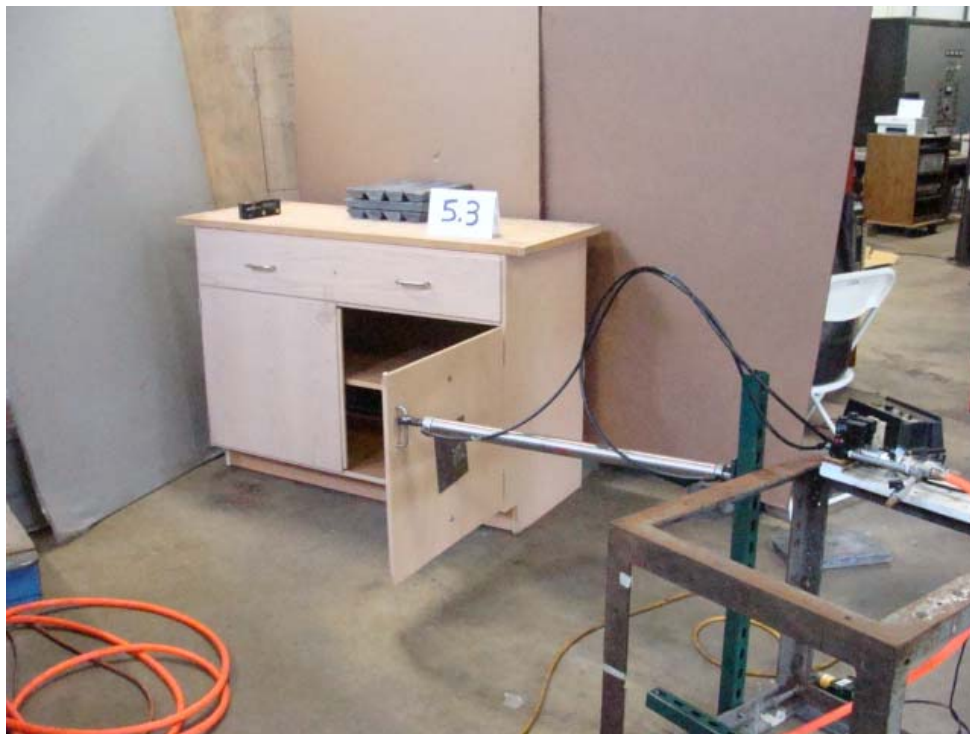
Photo 6: 5.3 Door Cycle Test
