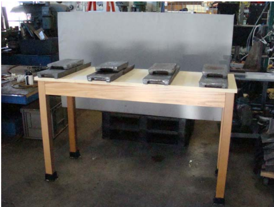
Photo 14: 10.2 Table Static Load Test
