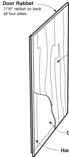
Door 3/4" 3-ply Composite Core Plywood Plain Sliced Face Veneer
