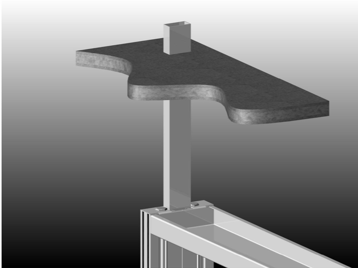
Once the ceiling extension tube is in the proper location. Drill and insert locking screw as shown.
