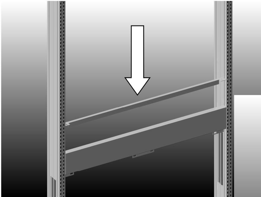
Be sure to leave 1/8" gap between the mounting bracket and the support bracket.
