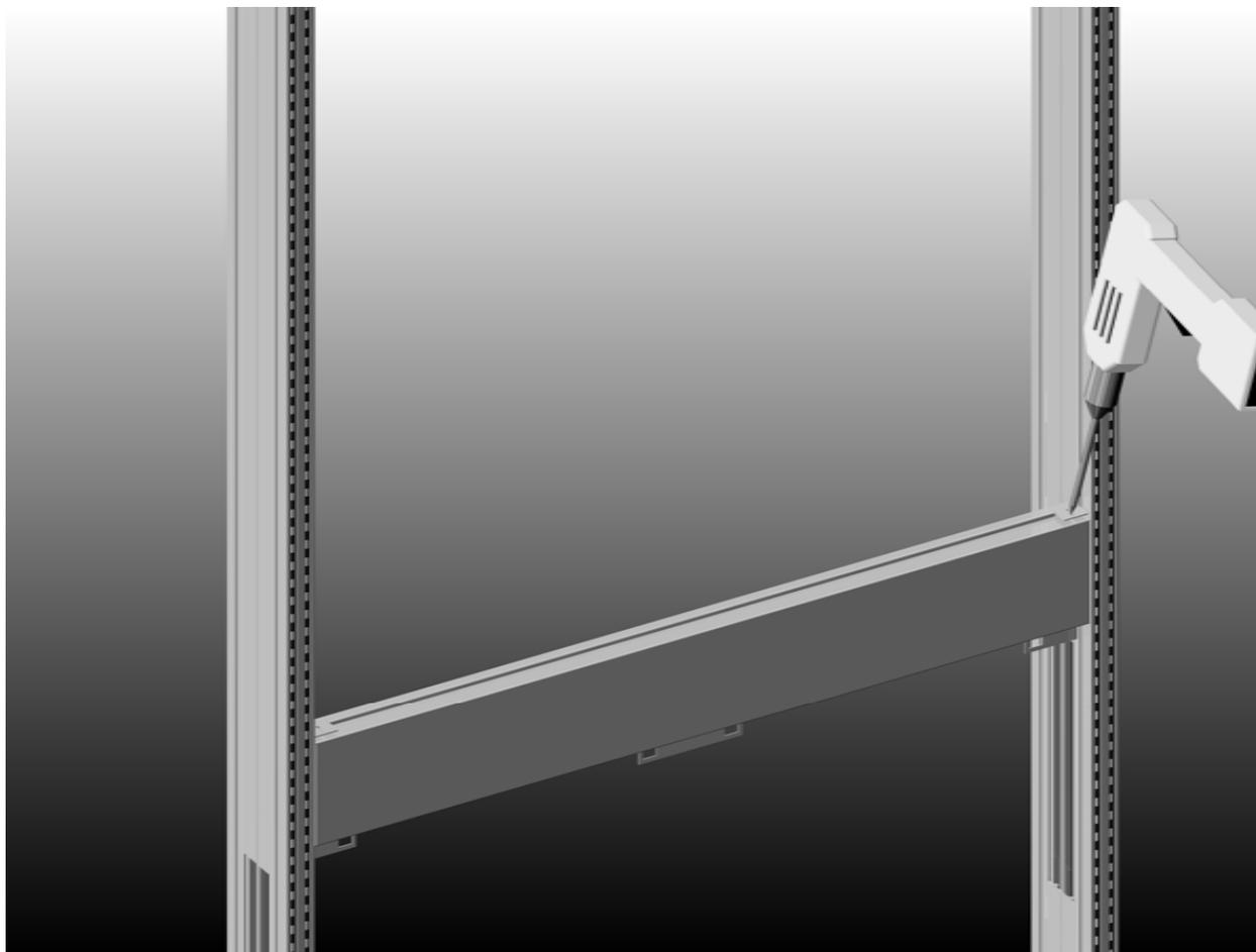
Insert the lower flange of the access panel into the slot between the panel mounting bracket and panel support bracket. Rotate the panel upward until the latching mechanism catches. The oversized punched hole in the panel and bracket allow for fine adjustment of the latch to correct misalignment.
