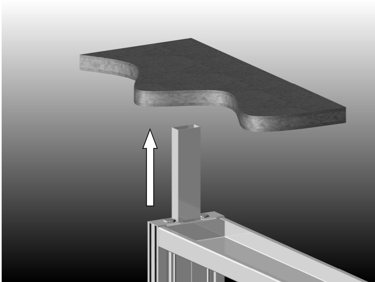
If the ceiling is suspended, cut a 1" x 2" opening in ceiling to allow the extension tube to protrude through the ceiling.
