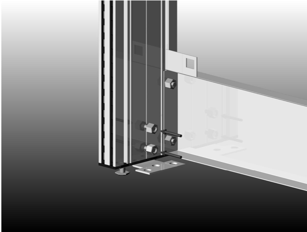
INSIDE PANEL NOT SHOWN TO DETAIL ANCHORING SYSTEM
