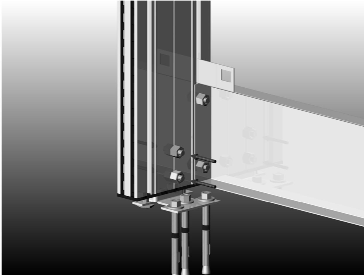
INSIDE PANEL AND FLOOR NOT SHOWN TO DETAIL ANCHORING SYSTEM
