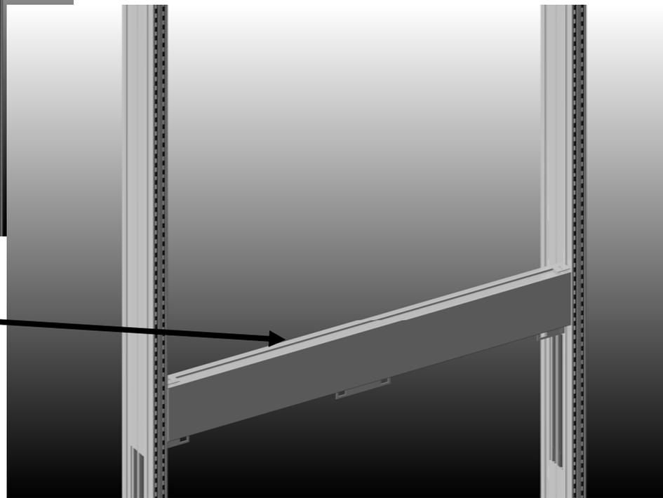
Drill and screw through the slot located at both ends.
