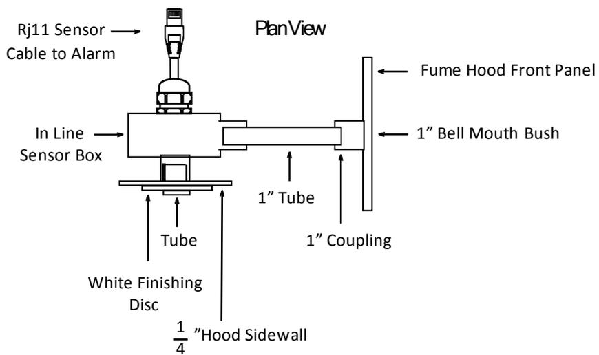
It is very important to position the SM6 airflow sensor in the correct position to give long term stable reading of the face velocity. Please read the INSTALLATION NOTES below and if in doubt contact us for further advice.
